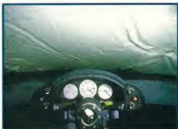
A FULL SHOT OF THE DASH, WITH THE SHEET ON THE WINDOW FOR CONTRAST WHEN CUTTING OUT.
